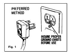
Have wall outlet and circuit checked by a qualified electrician to make sure the outlet is properly grounded. Where a standard two-prong wall outlet is encountered, it is your personal responsibility and obligation to have it replaced with a properly grounded three-prong wall outlet.
